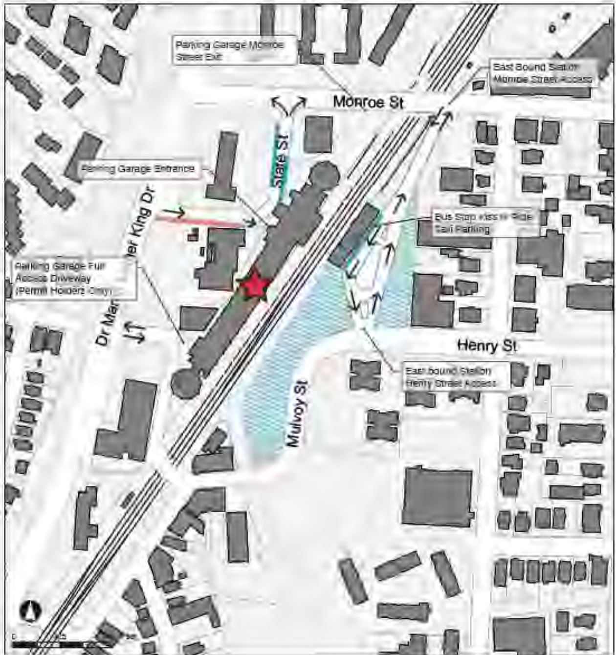
Figure 14: Train Station Access and Vehicular Circulation "Train Station Access and Vehicular Circulation" (Figure 14)
